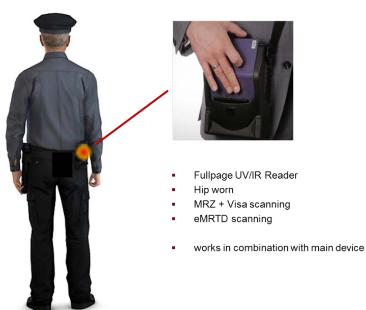
Figure 9: A2 - Full Page Passport reader without a display and long range communication functionality
