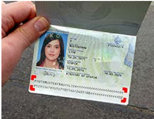
Figure 23: Red markers on the finder display show the calculated MRZ position
