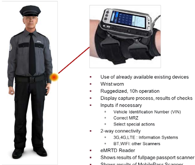
Figure 8: A1 - COTS ruggedized Devices with missing functionality, works in combination with additional elements
